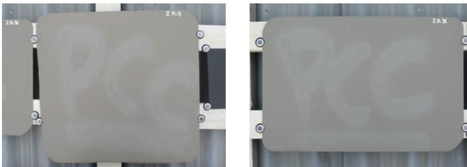
Fading effects of spray paint on ColorCote ZR8™ and ZRX™ – 18 months after installation
